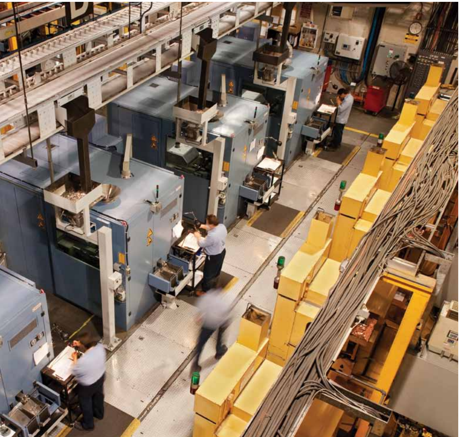
Over 40 high-speed coining presses produce up to 20 million circulation coins at the Winnipeg facility each day.
