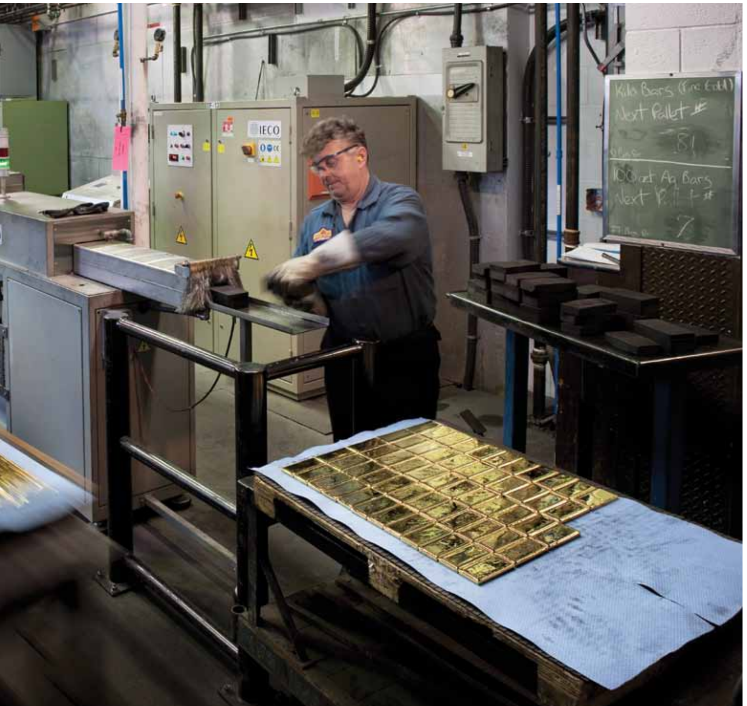
In operation since July, 2009 at its Ottawa facility, the Mint's high-speed bar-casting furnace produces 100-ounce silver bars and gold kilo bars.
