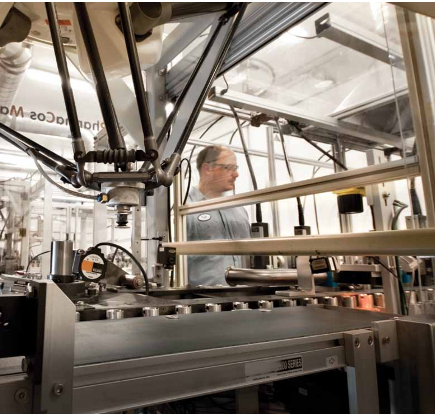
The Mint's robotic system for high-precision coin painting assists in satisfying specialty requests from foreign customers as well as special commemorative Canadian circulation coins.
