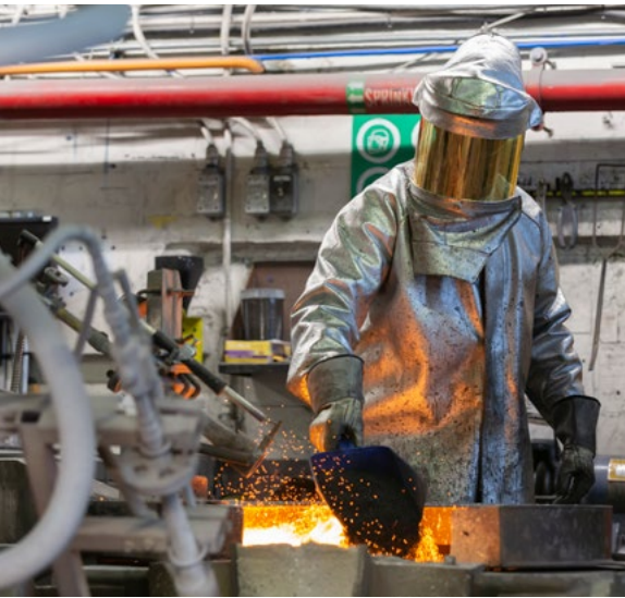
Top: Refined gold samples undergoing fire assay. Bottom: A refinery operator pouring pure silver bars at the Mint's Ottawa facility.
